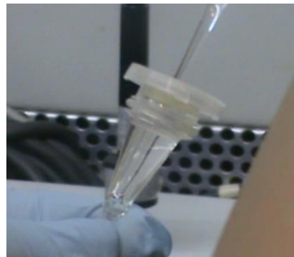
PICTURE 2: FILLING THE INNER CHAMBER WITH A PIPETTE FILLED WITH CULTURE MEDIUM
